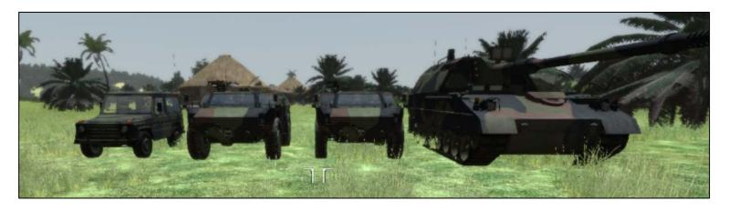
Results: weather conditions **do not have any influence** on vehicles' movement (only exception: 1,50m snow); **no groove tracks** on wet terrain; maximum speed of vehicles with tyres decreases from street to lawn/gravel to sand; **maximum speed of tracked vehicles does not decrease** due to terrain
